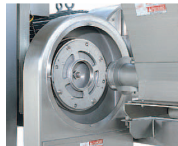
Cutting unit with cutting enclosure removed. (Shown for illustration purposes only)
