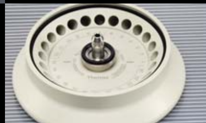
▶ 24 x 1.5/2.0 ml rotor with ClickSeal bio-containment lid
