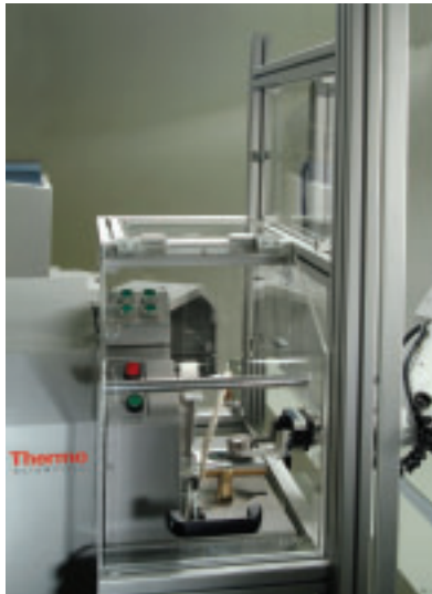
ARL 4460 robot access for automatic analysis
