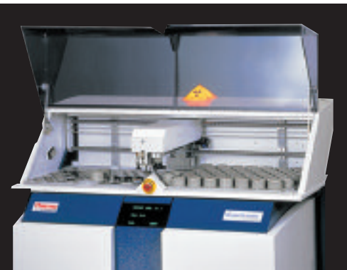
The large sample changer fits directly on top of the instrument
