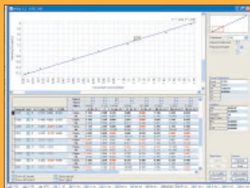
MVR calibration curve: real concentrations vs. intensities
