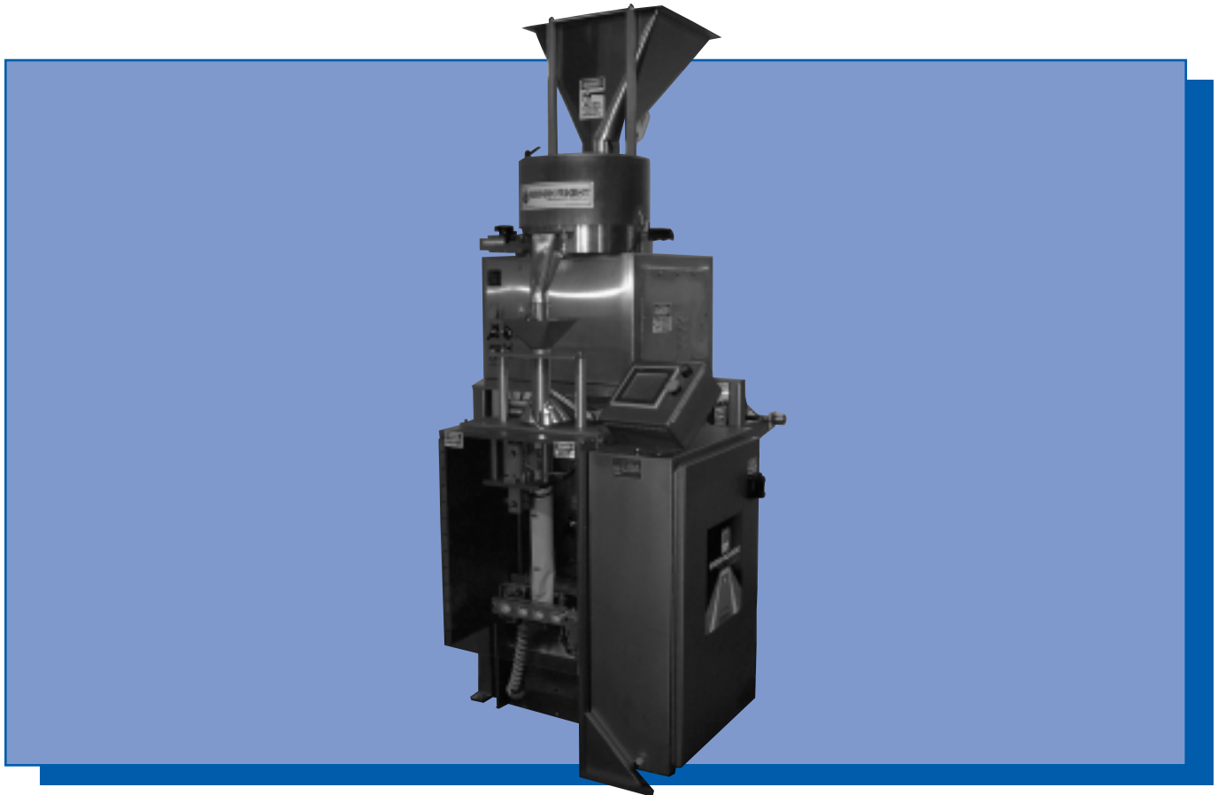
Machine is pictured with optional volumetric filler and thermal transfer printer.
