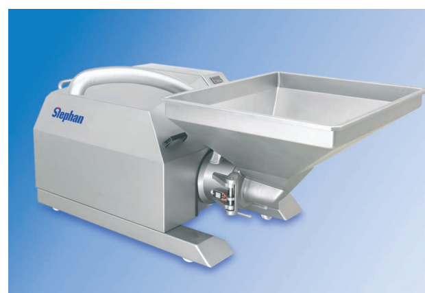
MCH a. MCH-D High-speed cutting and emulsifying of meat, fish and baby food
