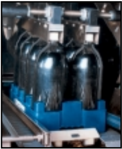
① Orbitron's technology advantage begins with the compact rotary product spacing wheel.
