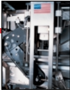
⑤ Direct drive "shear arm" assembly eliminates gearbox backlash for accurate bottle to case timing.
