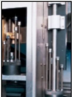
④ Positive positioning change part locators are provided with pre-set stops to allow immediate start-up and production.
