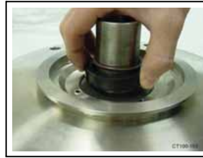
Figure 16 - Push Rotary Seal Down Releasing O-ring
