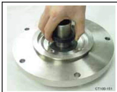
Figure 20 - Move Rotary Seal Up Shaft
