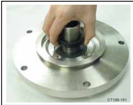
Figure 15 - Move Rotary Seal Up Shaft
