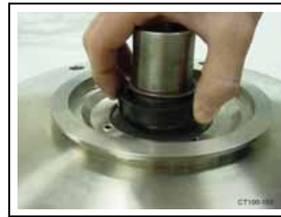
Figure 21 - Push Rotary Seal Down Releasing O-ring
