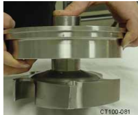
Figure 16 - Moving the Rotary Seal up the Shaft
