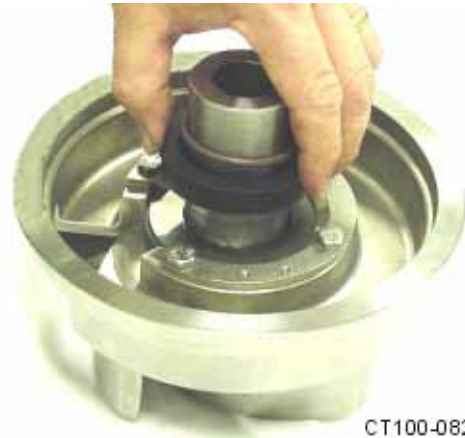
Figure 4 - Push Rotary Seal Down Until the O-ring is Released.
