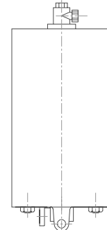
4" DIA ACTUATOR-AIR TO SPRING (1" THRU 4" SIZE VALVES.)
