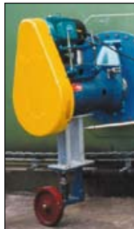
fig. 9: Castor Support on Belt Mixer
