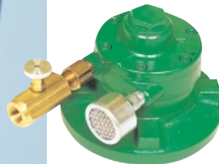
Optional 1/4 to 3/4 hp cool-running air motors can be used in flammable or explosive environments, and in ambient temperatures up to 250°F (120°C).
