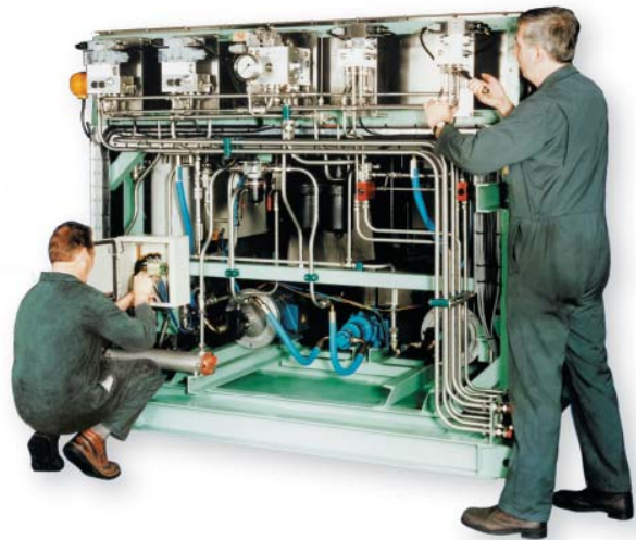
Typical skid mounted HPU.
