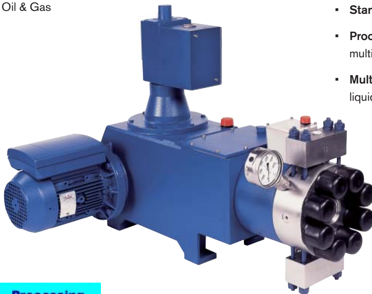
Metering pump type H4 with high pressure diaphragm pumphead and flow rate control via electric stroke length adjustment
