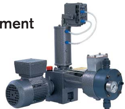
Metering pump type H1 with plastic diaphragm pumphead and flow rate control via pneumatic stroke length adjustment
