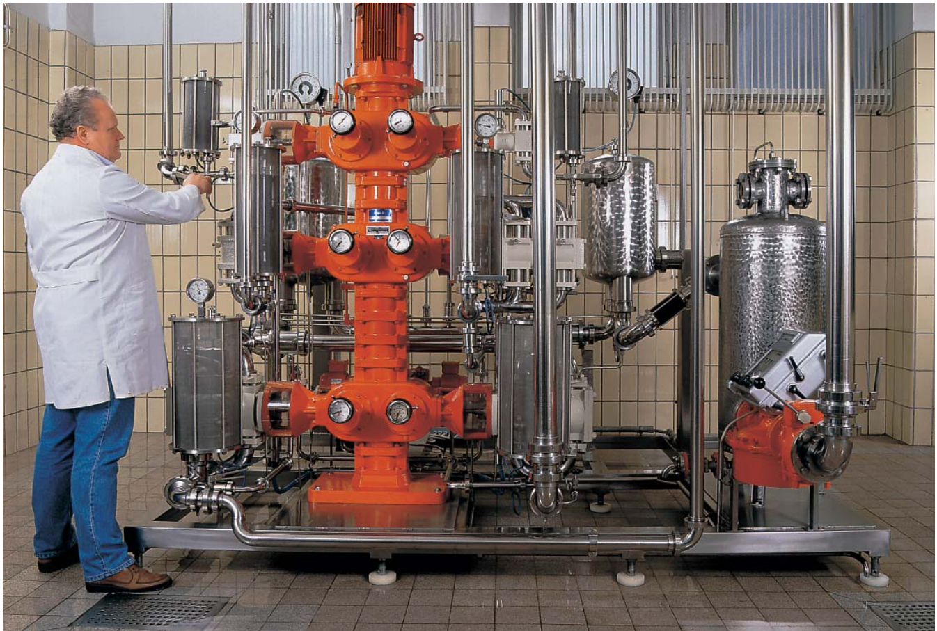
Continuous production of high-quality liqueur with multi-component metering and N-Form mixers.
