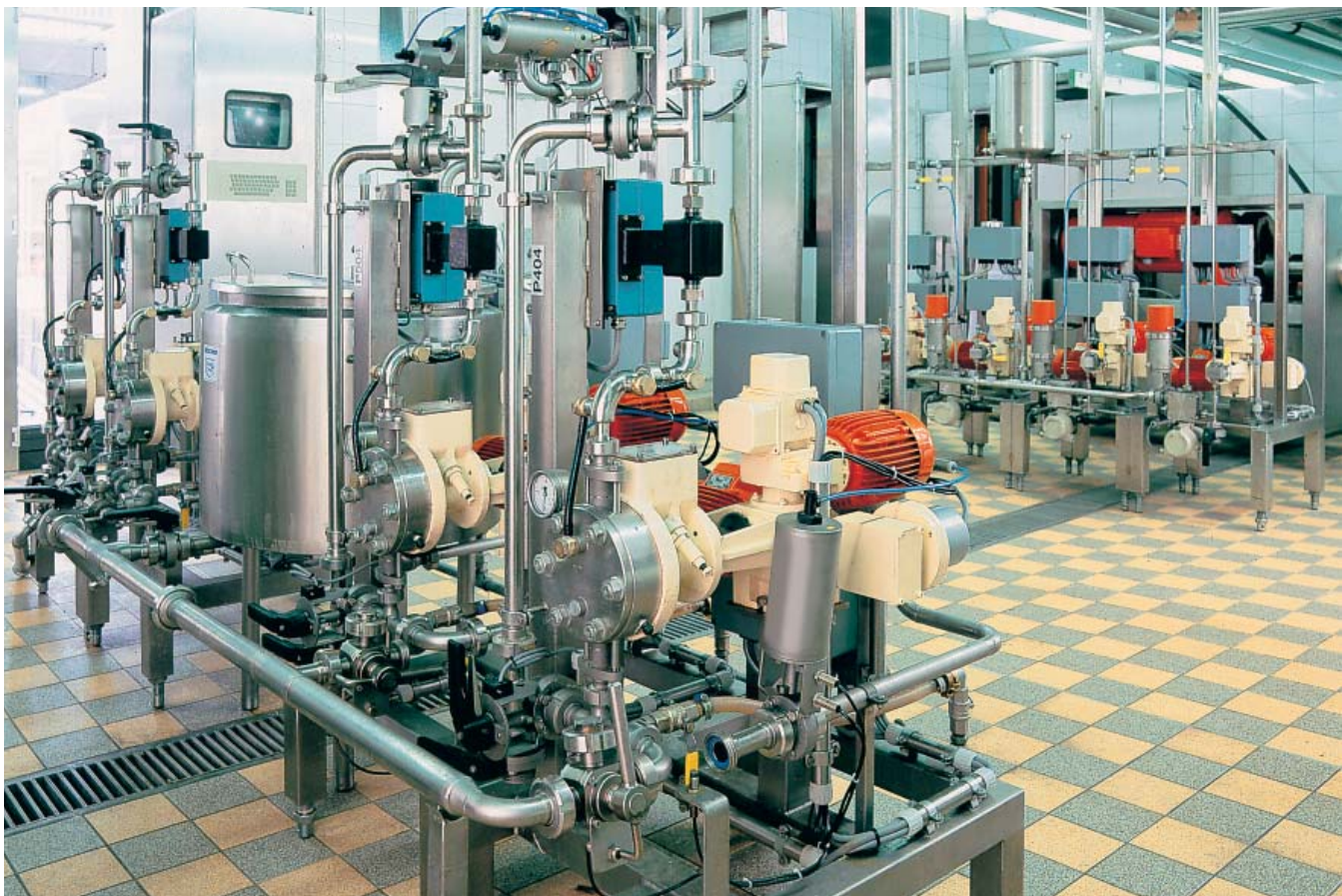
Installation for the continuous manufacture of aerated confectionery products, including metering pumps and flow measuring system.
