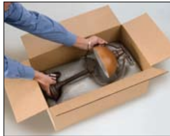
2. The Instamate® film is folded over, and the product is placed on the rising foam.
