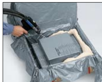
3. Instamate® film is placed into the mold, and Instapak® foam is dispensed.
