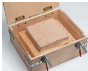
2. A simple wood mold is used to produce the desired cushion shape.
