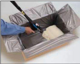
1. Instapak® foam is dispensed into a carton lined with high-strength Instamate® film.
