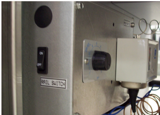
Figure 1 illustrates the electrical control box inside the mechanical compartment. The on/off switch for the rail is located on the front of the control box while the main on/off switch for the entire unit is located on the rear of the control box. The thermostat adjustment knob for the upper rail is located on the side of the control box.
