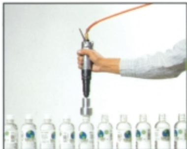
Norland's optional bottle cap tightener for smaller bottles will handle between 500 and 750 "flat-top" or "sports-top" caps per hour.
