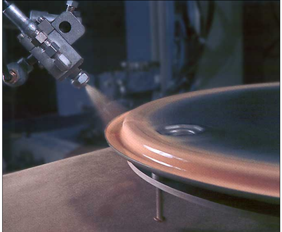
A7A guns are used on high-speed drum painting lines to deliver fast, precise coating coverage.
