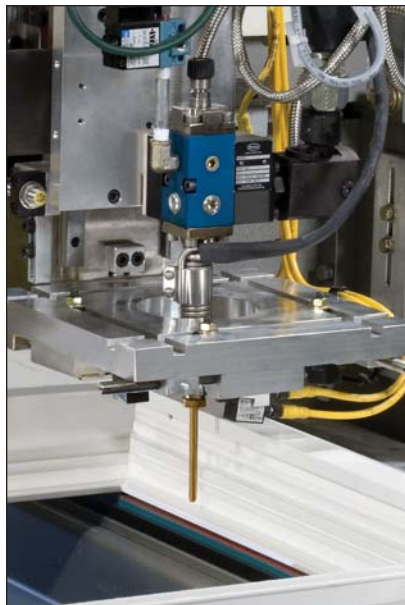
AG-900+ dispensing applicator in window backbedding application
