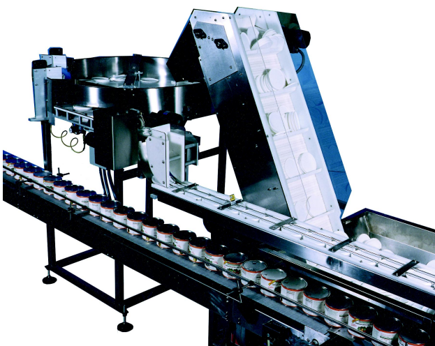
Additional cap sorter with optional airveyor
