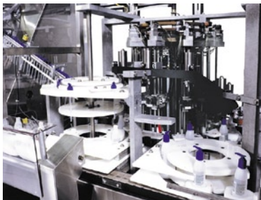
Close-up of pump placer area
