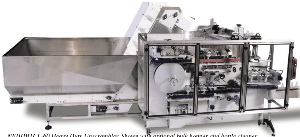
NEHHBTCL-60 Heavy Duty Unscrambler. Shown with optional bulk hopper and bottle cleaner
