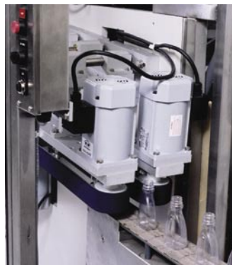
Integrated AC drive motors
