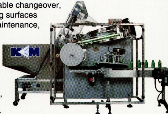
The NEHE with NEM 20 cu. ft. hopper elevator and guarding frame shown.
