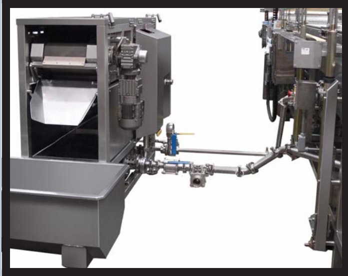
Filter Connected to Fryer
