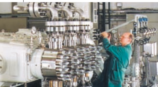
LEWA triplex process diaphragm pumps
