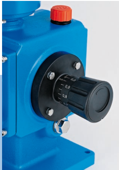
Linear stroke adjustment at the hand wheel in stages of 0.05 mm is possible both at standstill and during operations.
