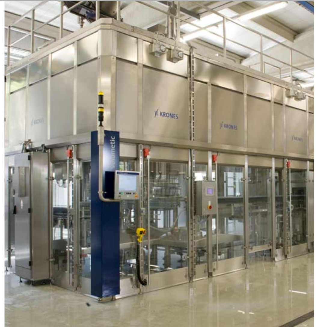
Clean room housing
