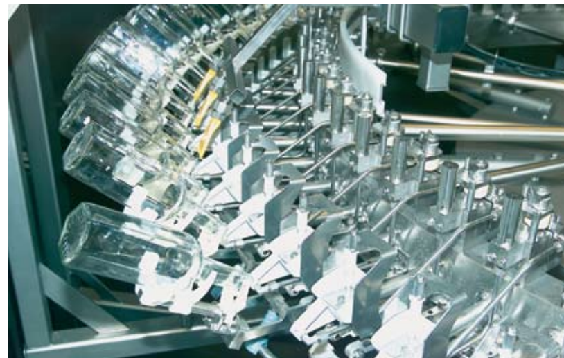
Nozzle unit of the single-channel rinser for ionised air (picture top left)
