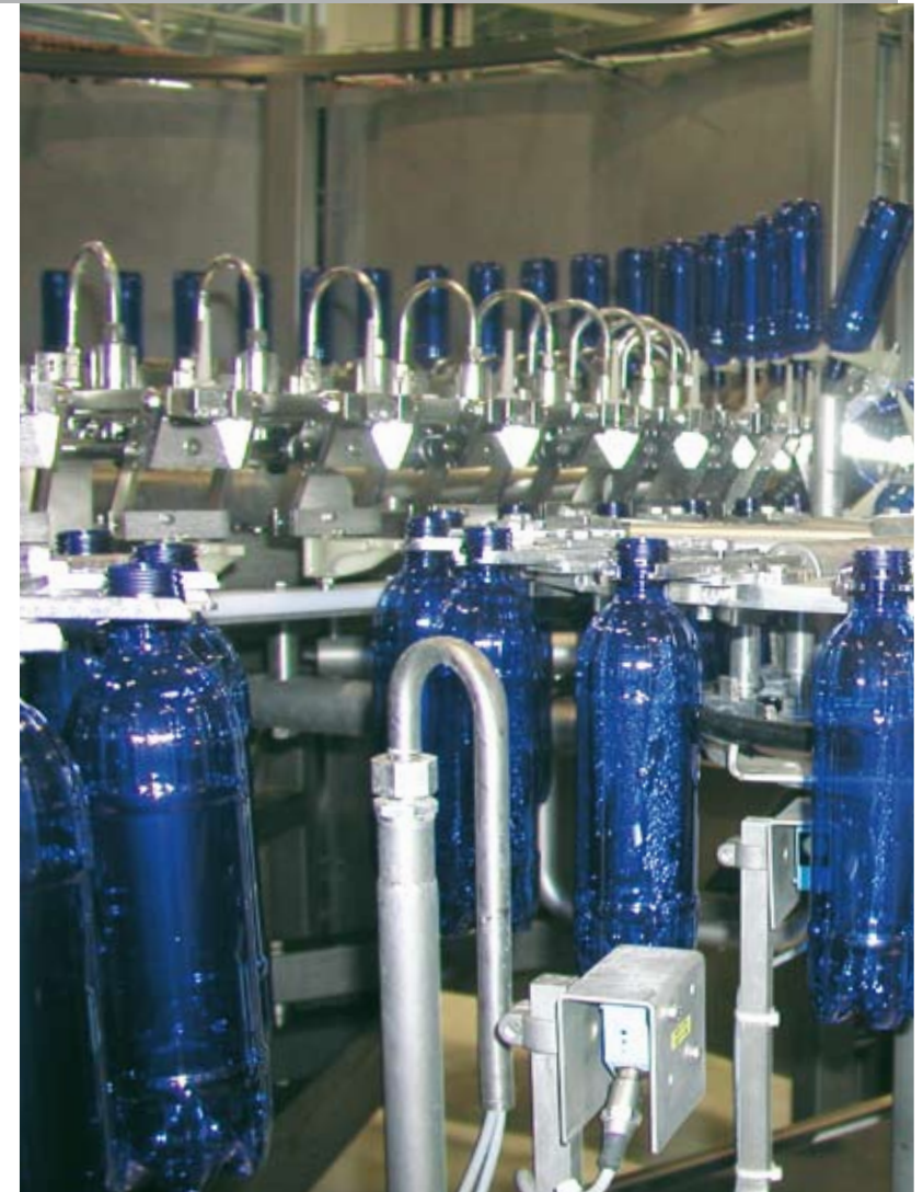
Variojet two-channel rinser for PET bottles
