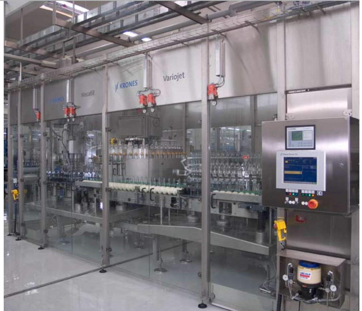
Bloc with the Variojet rinsing station and the Mecafill VKP filler in a gable-type table top arrangement
