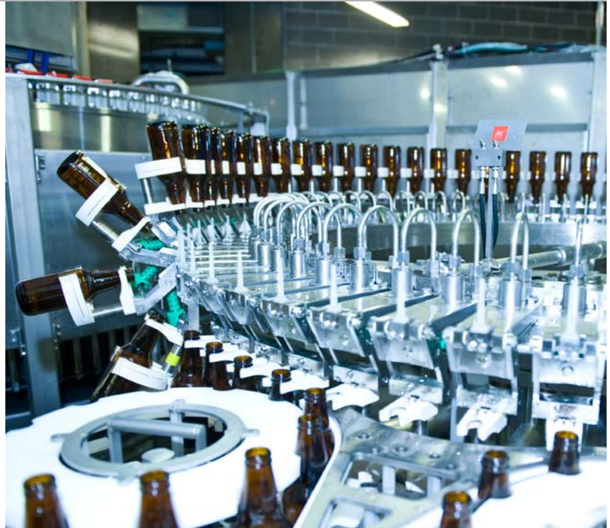
Mechanical single-channel rinser Variojet for glass bottles
