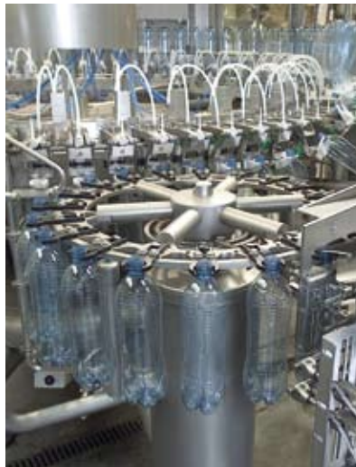
Rinser with free-standing Monotec starwheel column
