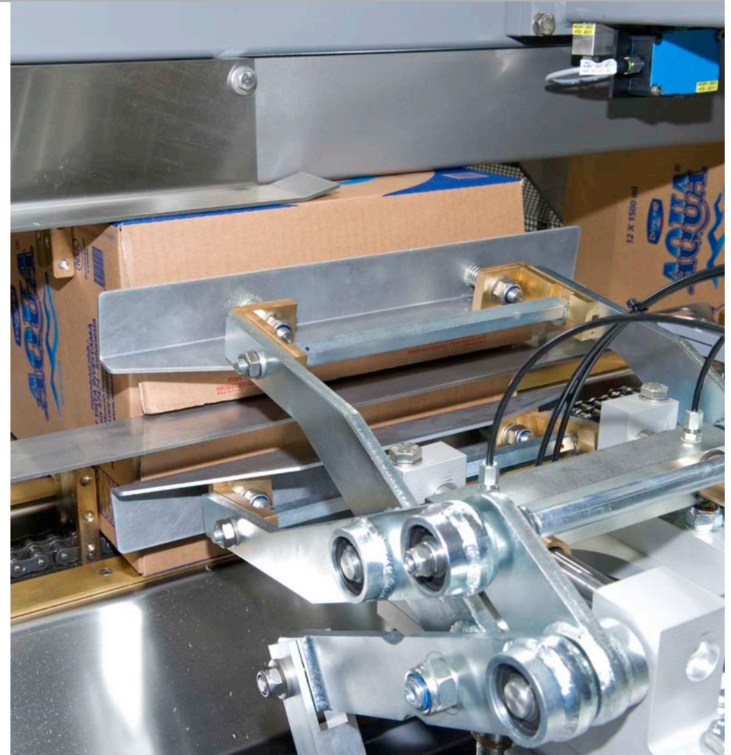
Folding in the side flaps on the closing station
