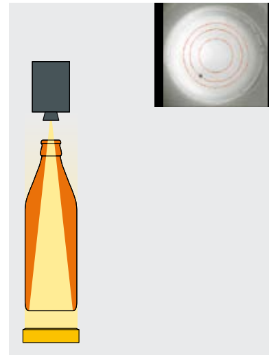
Base inspection unit
