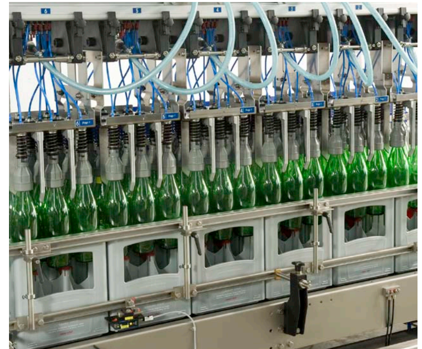
Rigid gripper head for removing glass bottles from returnable packs
