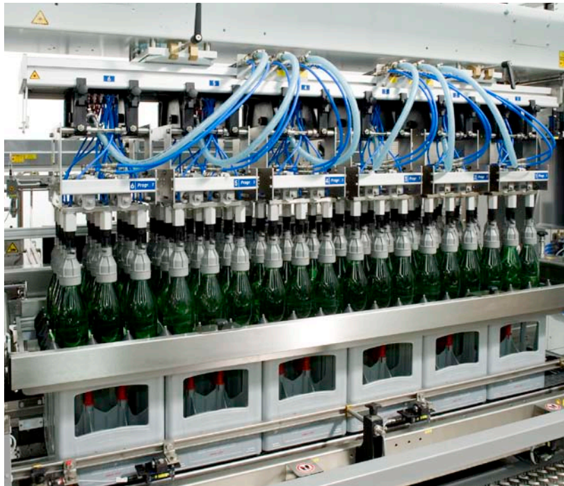
One-dimensional, flexible gripper head for precise insertion into packs
