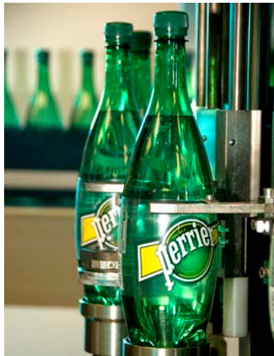
Sleeve transfer with the Sleevematic AF
