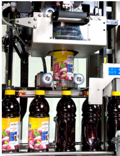
Sleeve transfer with the Sleevematic M
