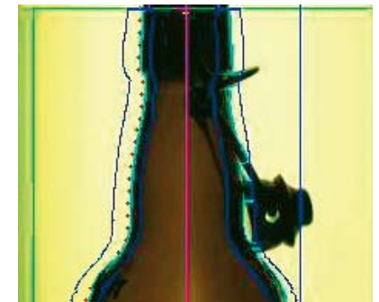
Example of contour detection with different glass bottles
