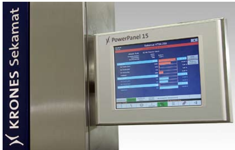
The Sekamat can be operated easily and safely via touch-screen.
