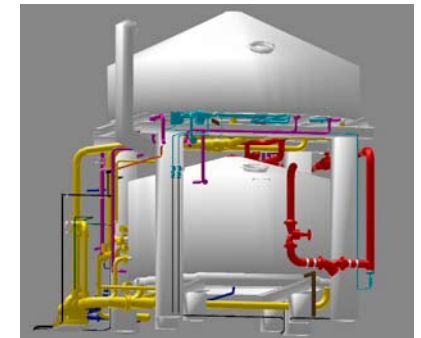
Example of the pipe system with Merlin above Whirlpool
