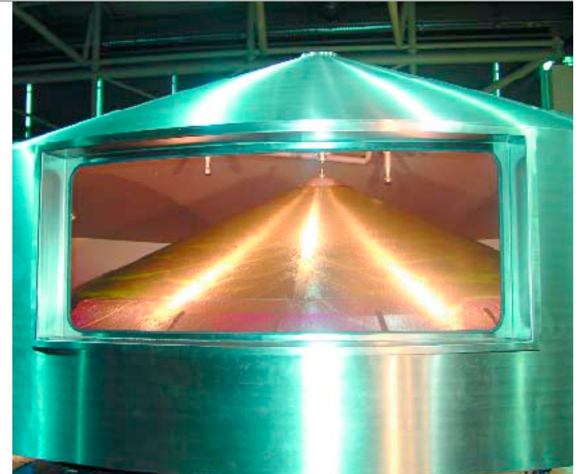
Merlin wort boiling and stripping system
