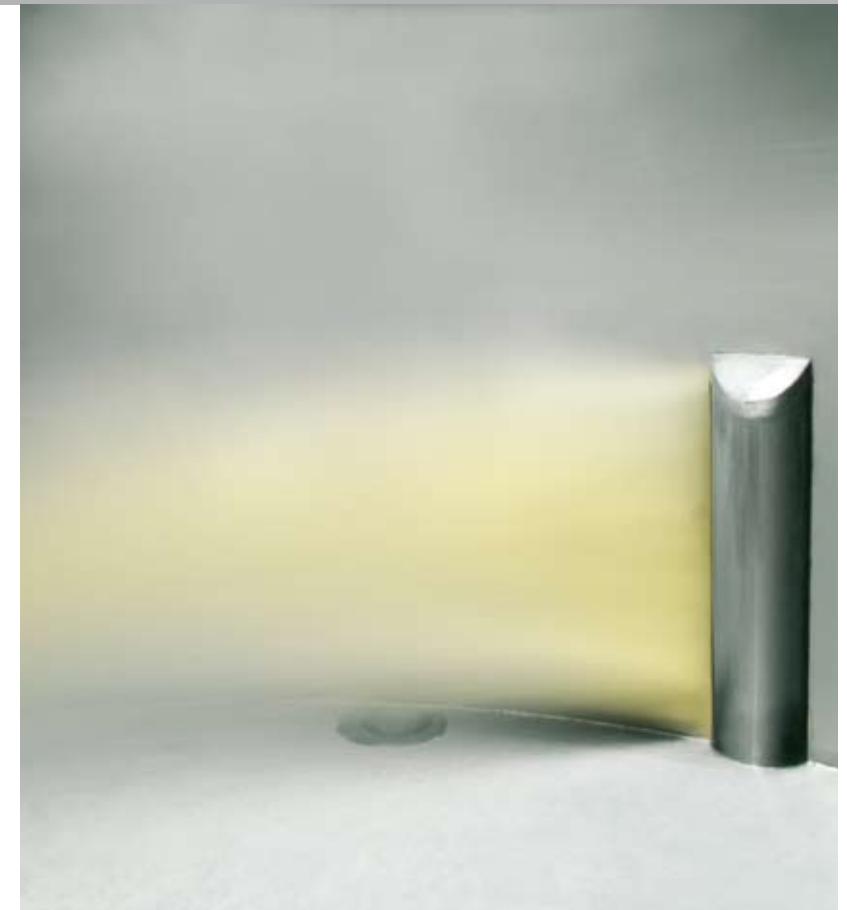
The wort enters the whirlpool in an even, widely fanned jet
