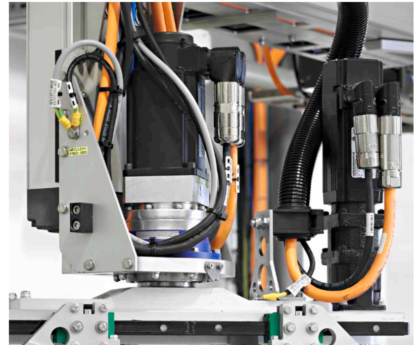
Compact and easily accessible: the turning unit above the gripper head
