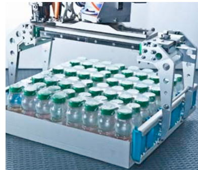
The gripper heads with plastic fins guarantee gentle pack handling.
