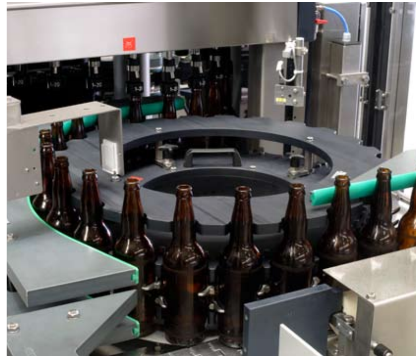
Retaining bar starwheels
