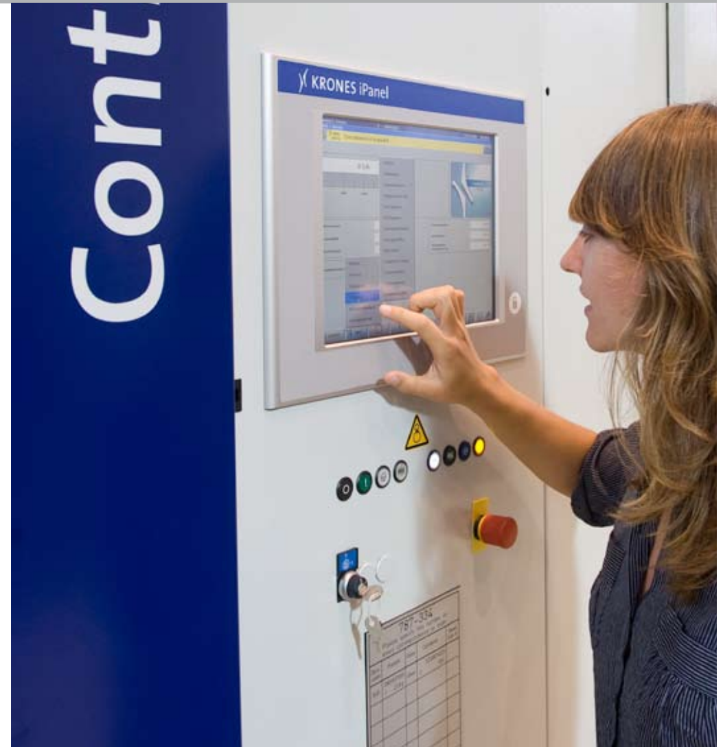
Operation of the stretch blow moulder is from the central touch-screen.
