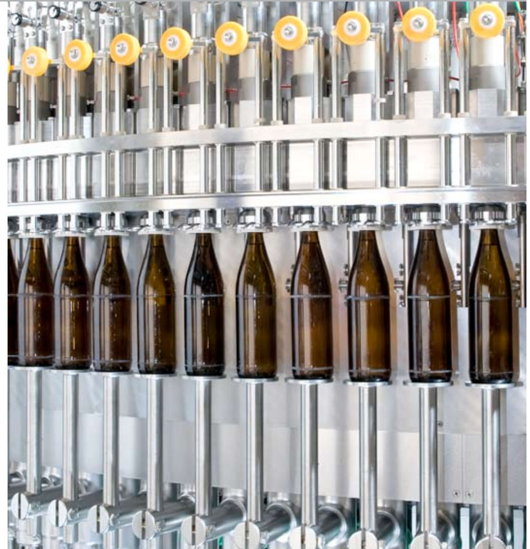
Filling valves in the Modulfill VP
