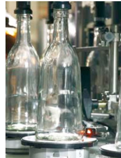
Mechanical container orientation via spotting bars on the side-wall (left picture)
