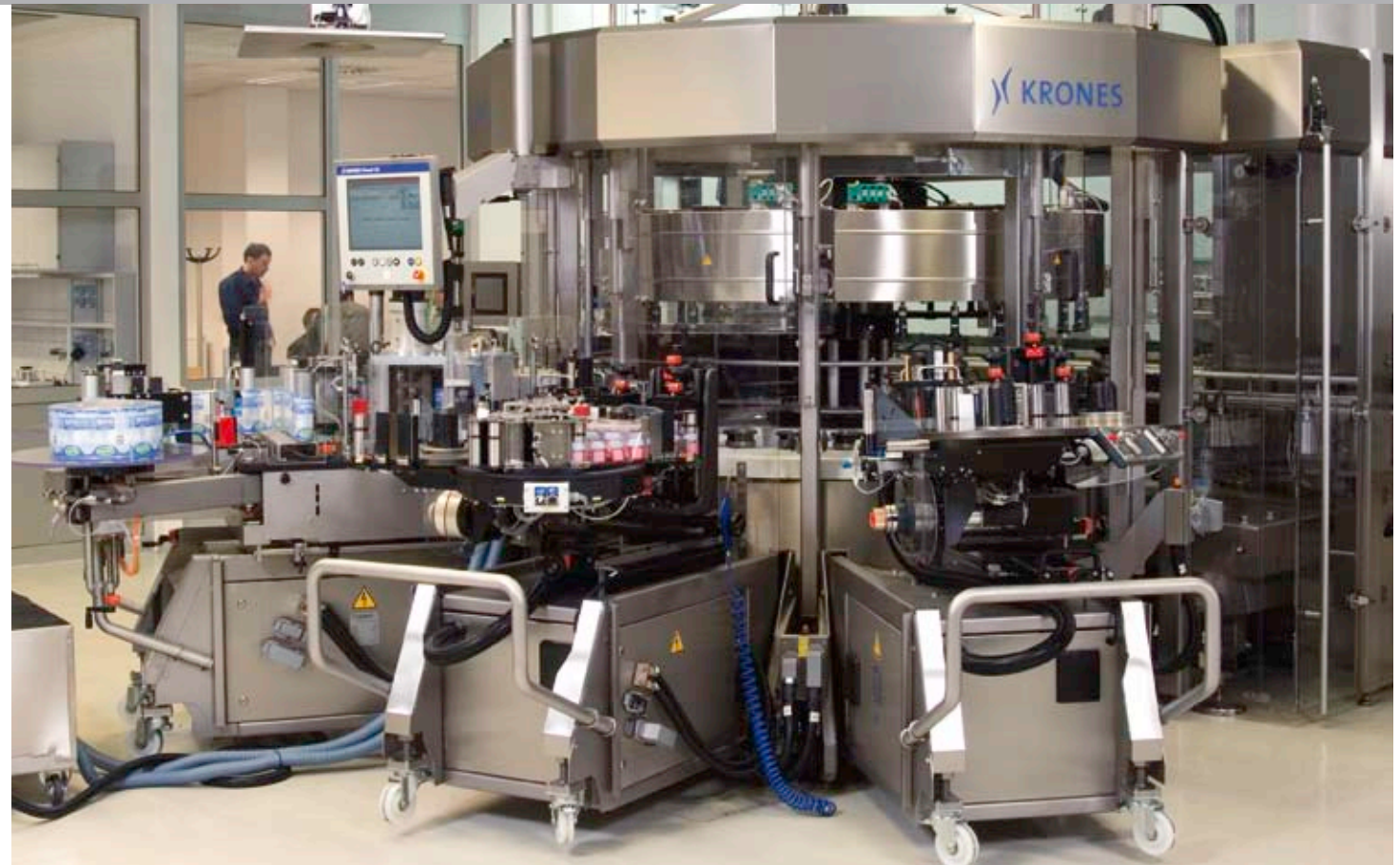
Topmodul with one Controll labelling station (left) and two self-adhesive labelling stations
