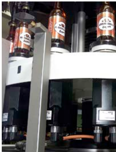
Container table with servomotors, protection type IP65
