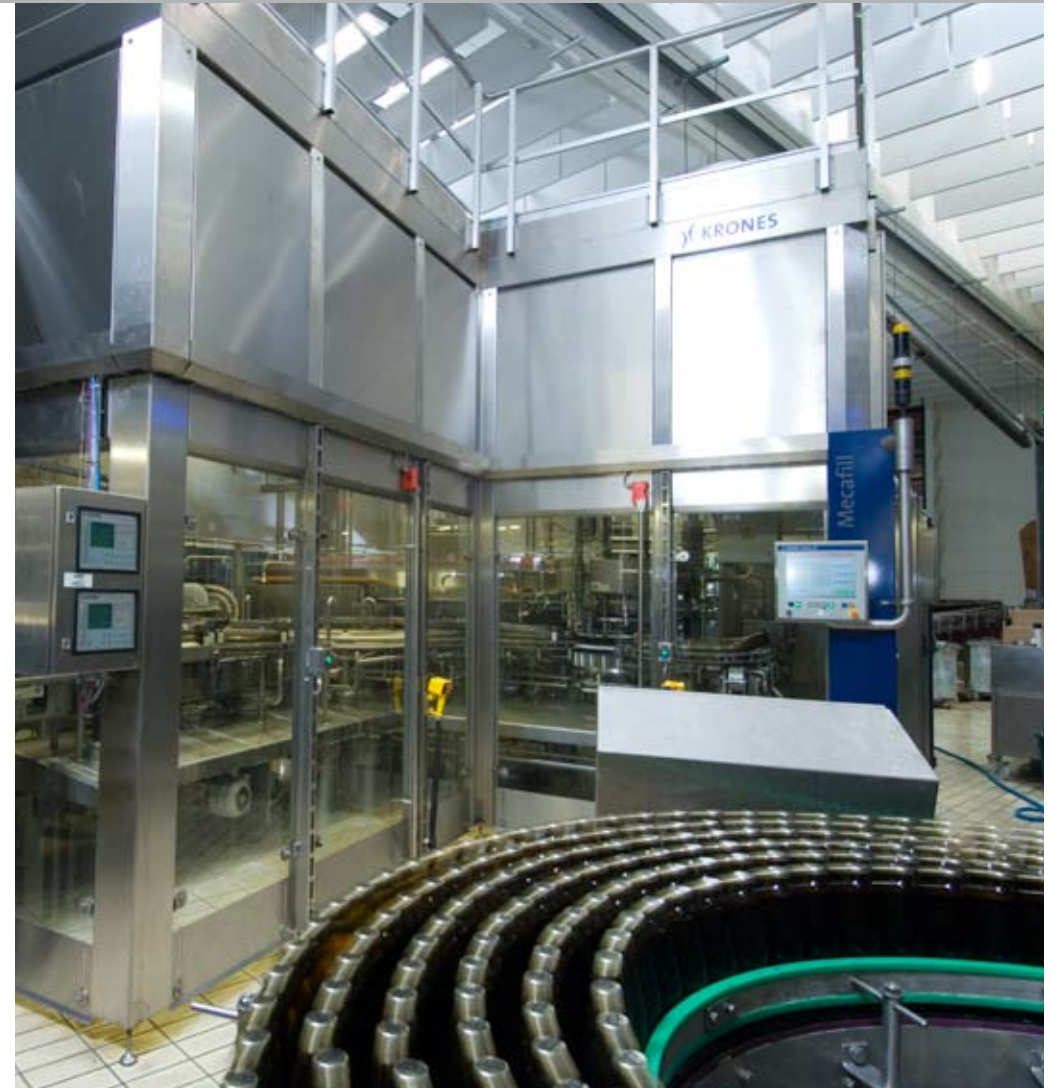
Clean room housing
