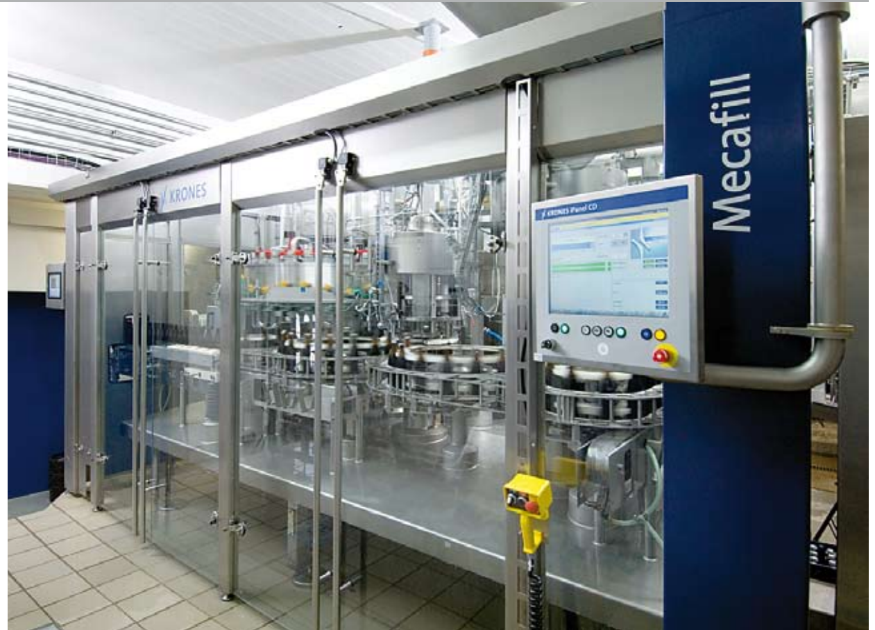
Mecafill VKPV-PET with gable-type table top design
