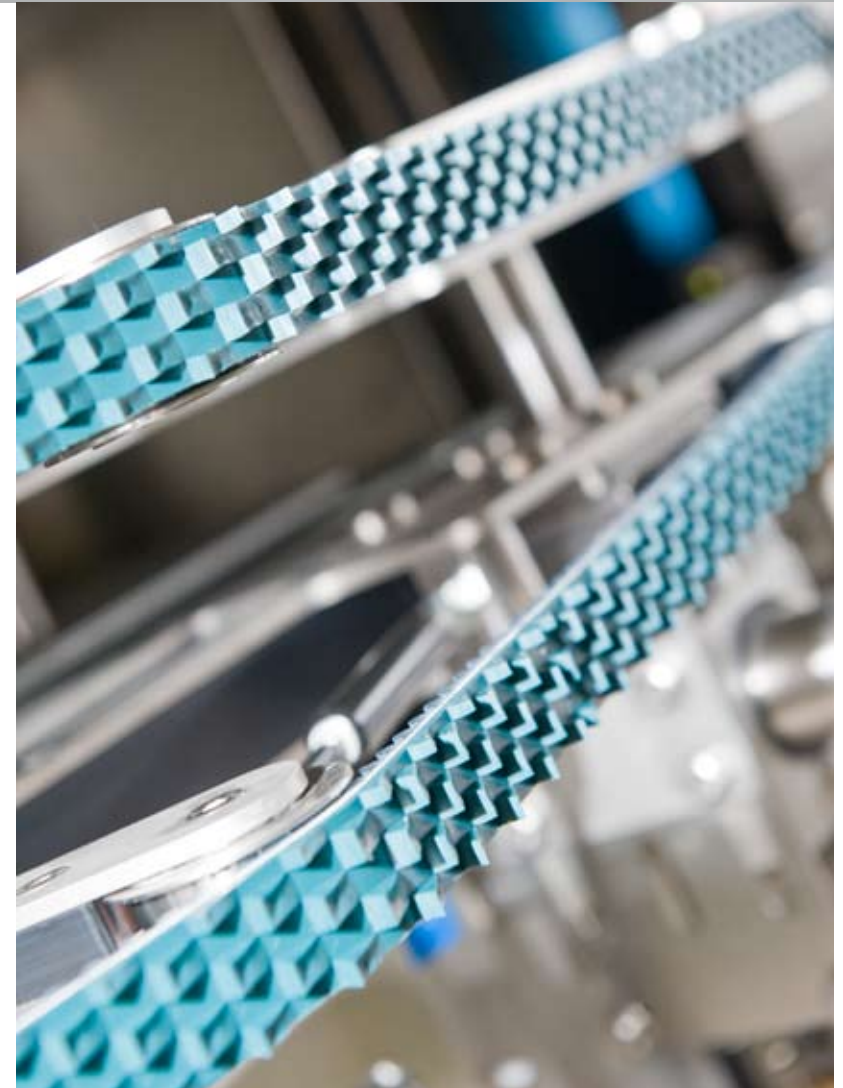
Container guidance by adjustable belts
