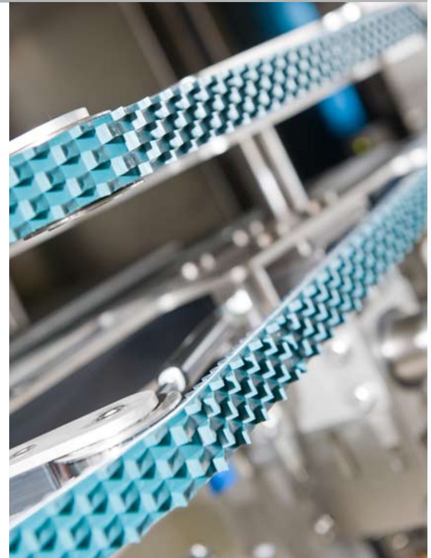
Container guide with adjustable belts
