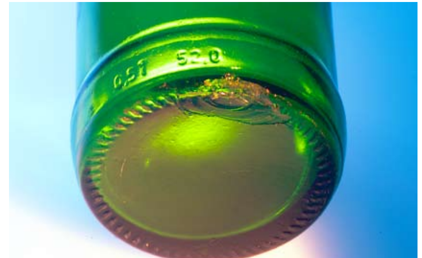
Chip on the container base
