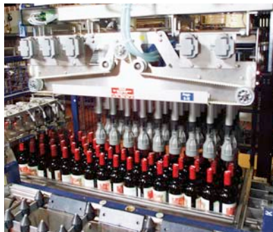
Spindle-adjustable gripper head for handling different container diameters
