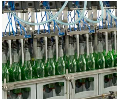
Rigid gripper head for removing glass bottles from returnable packs
