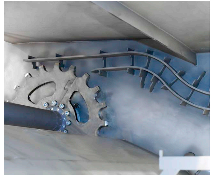
Split sprockets facilitate maintenance.
