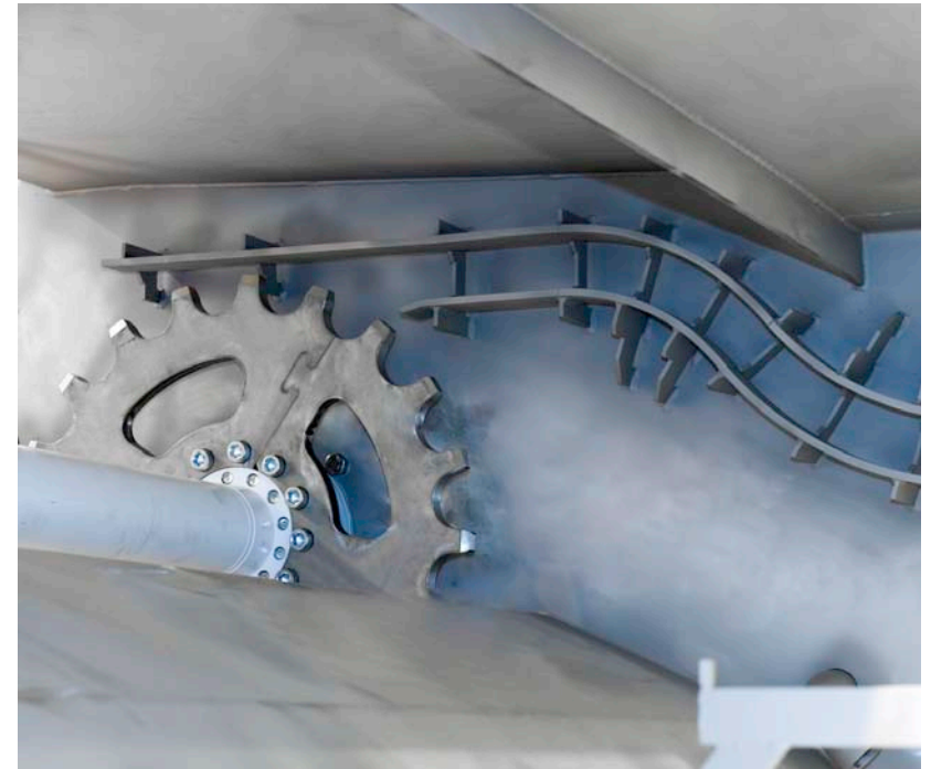
Split sprockets facilitate maintenance
