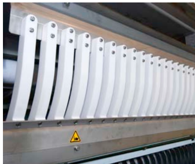
Open bottle chute made of plastic sections
