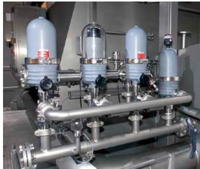
Combined coarse and fine filtration
