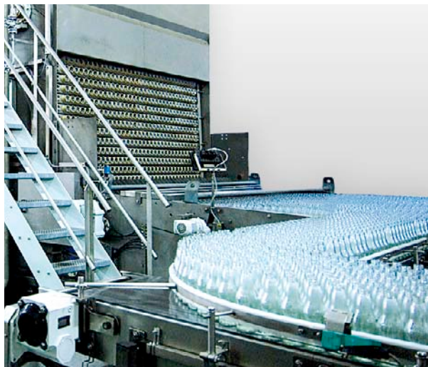
Designed as rinsers for non-returnable bottles
