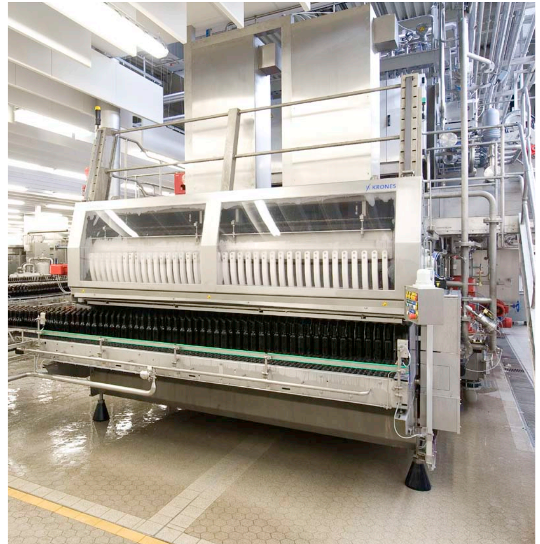
Combined coarse and fine filtration
