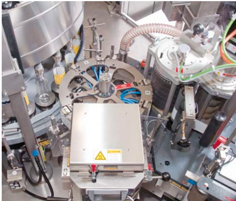
Labelling station with replaceable hotmelt gluing unit
